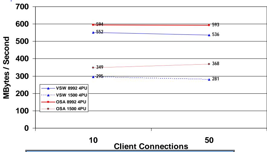
Using jumbo frames increases throughput between 61 to 91%.
